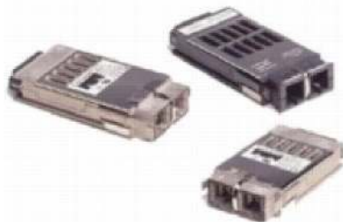
Figure 3. GBIC Transceiver Modules for the Cisco ONS Family
