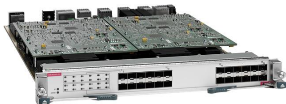
Figure 1. Cisco Nexus 7000 M2-Series 24-Port 10 Gigabit Ethernet Module with XL Option
