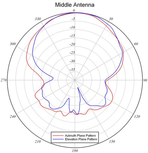
**Azimuth and Elevation Radiation Patterns**
