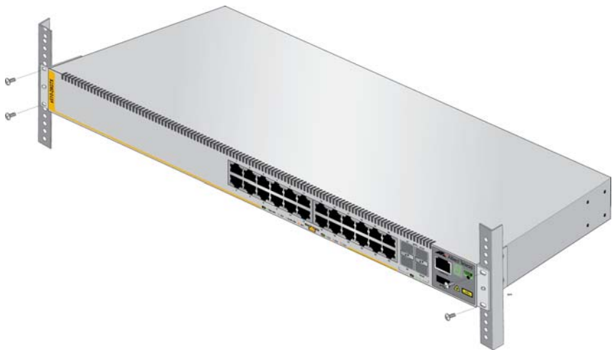
Figure 20. Mounting the Switch in an Equipment Rack
