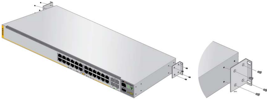
Figure 19. Attaching the Equipment Rack Brackets (Continued)
