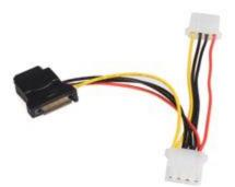
The LP4SATAFM2L SATA to LP4 Power Cable, lets you power an IDE (LP4-connected) drive using a SATA power connector from the computer power supply. The adapter features two additional LP4 power connectors, offering the versatility to connect two additional (LP4 connected) drives (CD/DVD-ROM, HDD, etc.) using the same single connection to the computer power supply.
