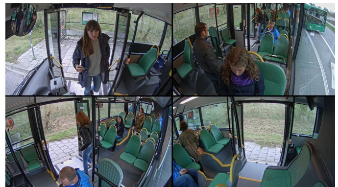
At left, an illustration with AXIS F44 (and local storage on SD cards), AXIS F1005-Es and a microphone in a bus. At right, quad view from a bus.
